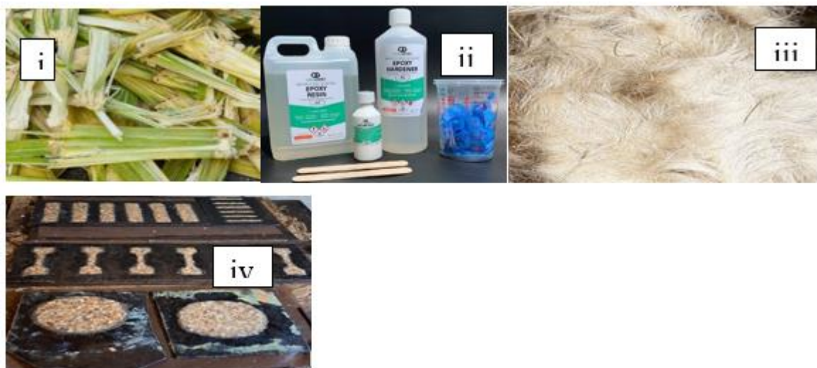
Figure 1: Sugarcane bagasse:(i). Epoxy resin and hardener (ii). Cow hair (iii). Cow bone (iv). Cow bone particulate
